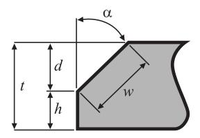
$\alpha$  = bevel angle d = bevel depth h = root face w = bevel width
